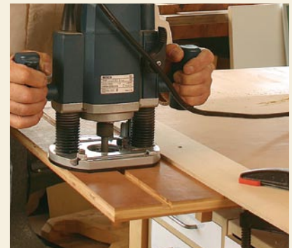
Cut clean and accurate dados. Clamp the dado jig at both ends and make the cut in two or three passes.
