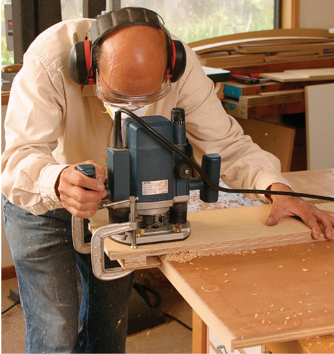
Flush-cut edge-banding. This jig allows you to cleanly cut solid-wood edge-banding flush with the plywood panel.
