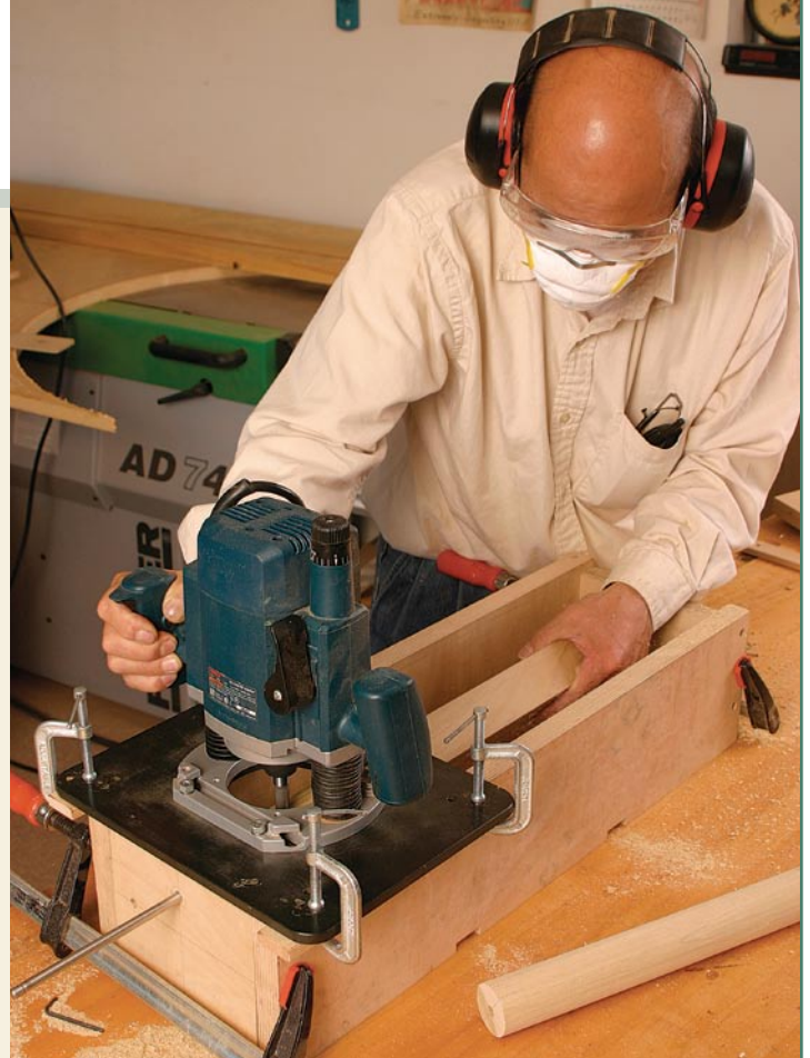
Router-cut turnings. By guiding the router back and forth while turning the workpiece, a square blank gradually becomes a cylinder.
