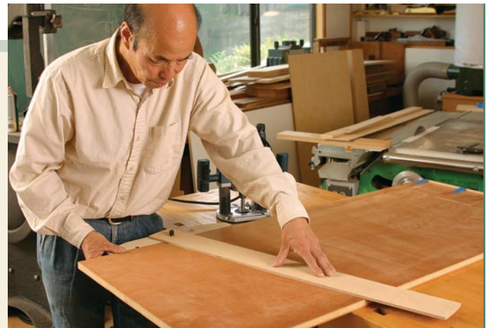
Variable-angle jig. Although dados usually are perpendicular to the long edges of a panel, this jig can make cuts at other angles.
