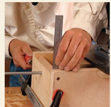
Tapered turnings. Lower the hole at one end of the jig to taper the turned workpiece.
